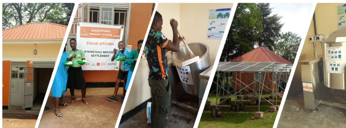
Kyangwali Primary School Kitchen, Uganda, using tilttable 110L induction stoves © Pesitho
